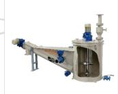
High-consumption lime industry use Dynemix lime slaker to convert hydrated lime or raw lime into lime slurry. Typically, a Lime slaker is comprised of two chambers. The first chamber is called the slaking chamber and the second chamber is usually used as a grit removal chamber.
