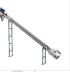
Drag chain conveyors work on the Principle of a chain-and-flight combination pulling a volume of material along. The chain is equipped with different flights/paddles and drags the material from various charging points to a number of discharging points.
